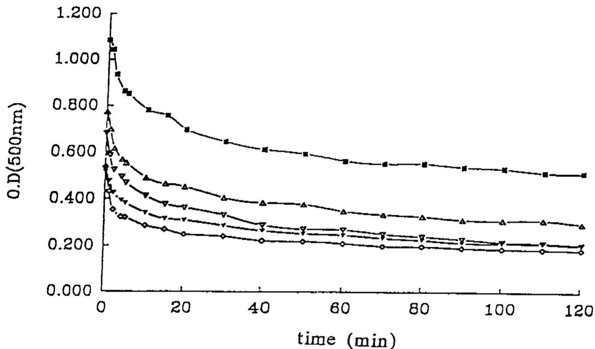
Fig.6 Change in turbidity of emulsions prepared using protein and oil at different ratios during setting.
