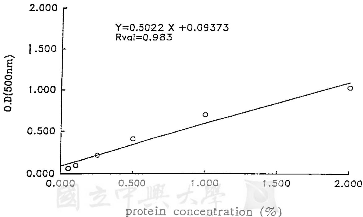
Fig.5 Emulsion capacity expressed using the slope of emulsion turbidity as a function of protein concentration.
