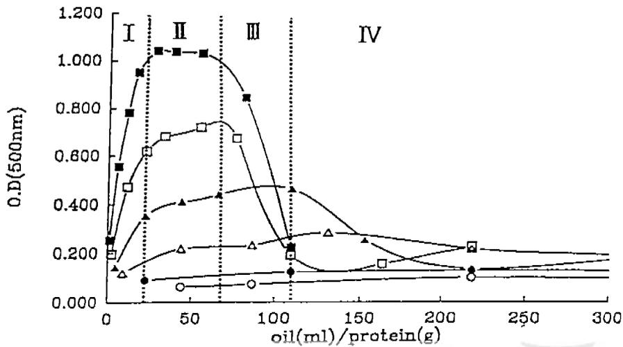
Fig.4 Effect of protein concentrations on the turbidity of emulsions prepared using protein and oil at different ratio.
