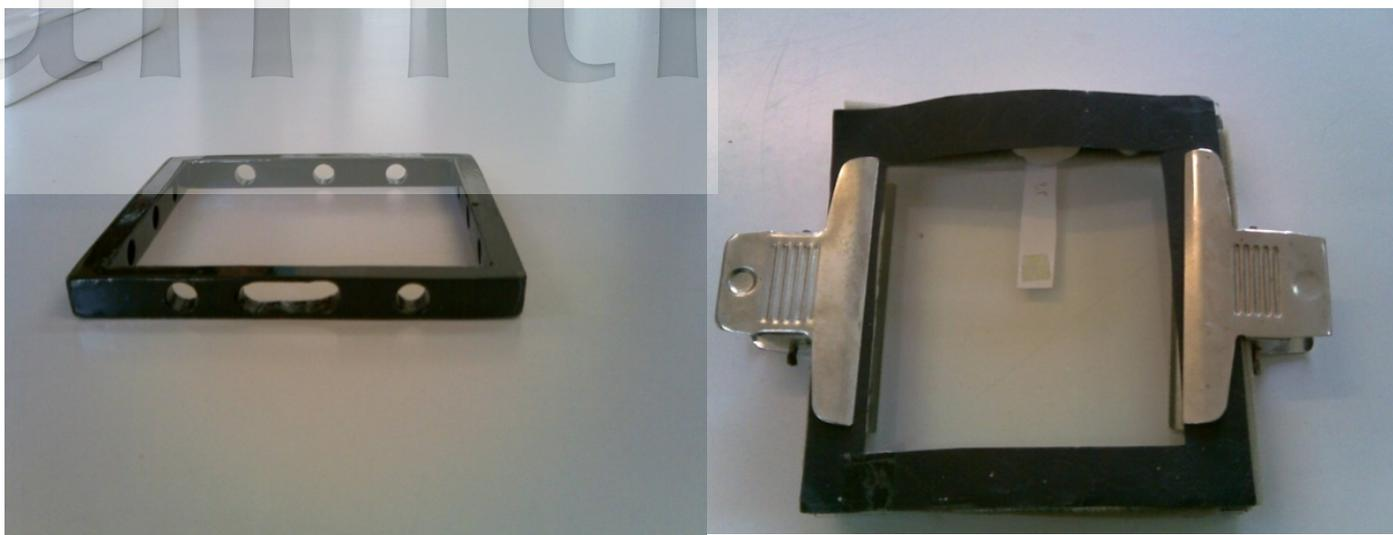
Fig. 1. The black colored aluminum frame (left) and prepared adult exposure cage (right)
